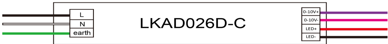
产品接线示意图/ Product Connection Diagram
